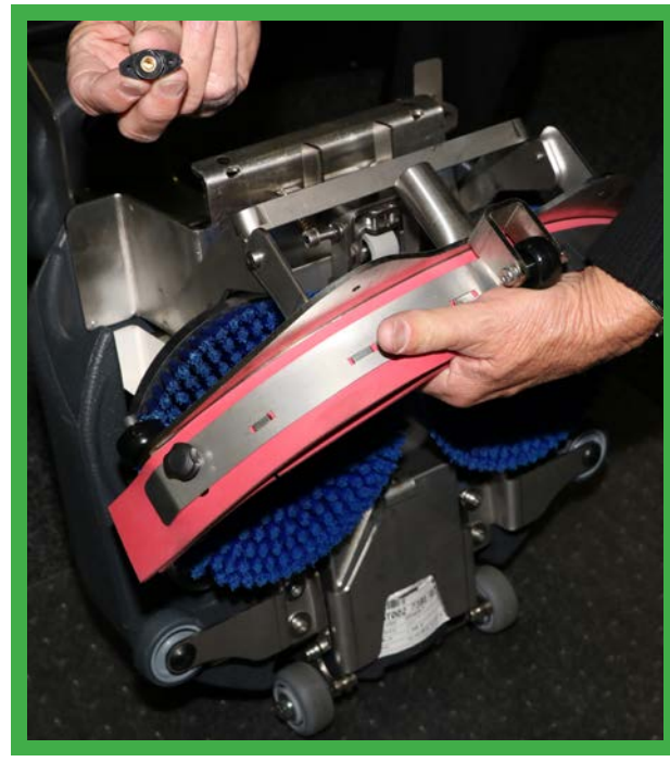
2. FIT SQUEEGEE ASSEMBLY WITH TWO WINGNUTS SUPPLIED
