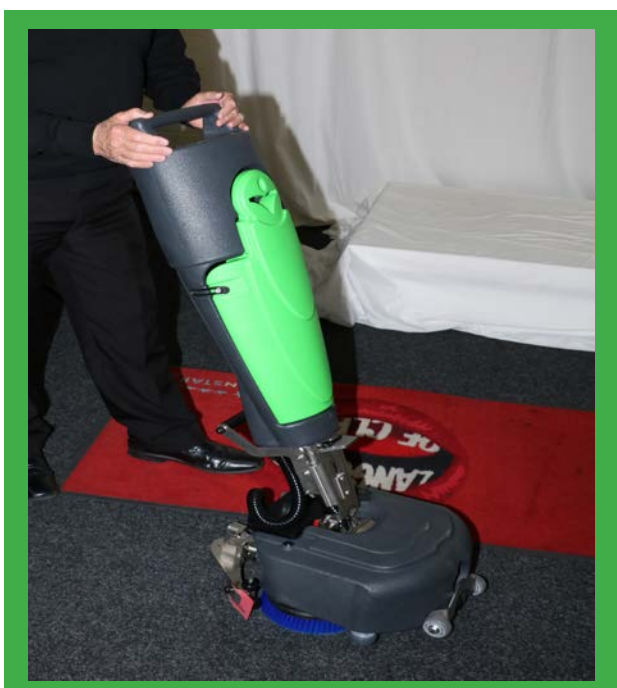
16. MAKE SURE MACHINE IS ALWAYS MOVING FORWARD, SQUEEGEE NEEDS TO FOLLOW BRUSH
