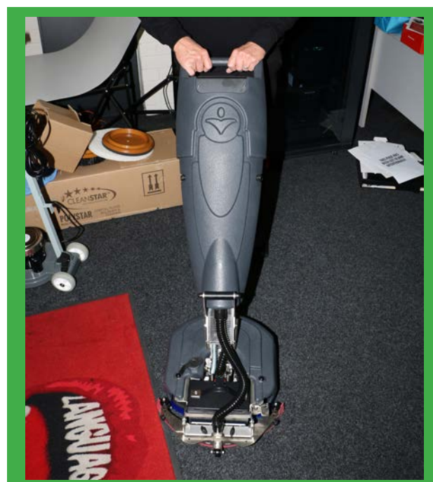
17. IF YOU WANT TO BRING MACHINE BACK TO YOU, ROTATE HANDLE AND PULL TOWARD YOU.
