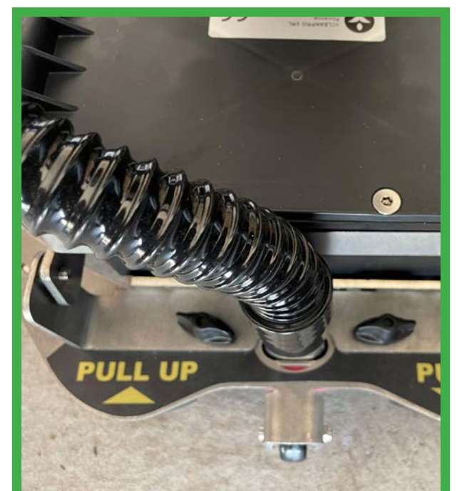
20. 'PULL UP' TO LIFT THE SQUEEGEE ASSEMBLY
