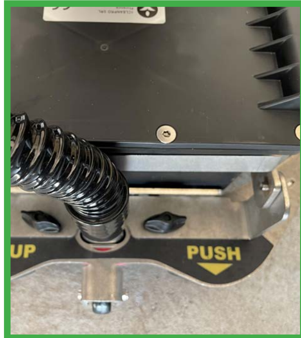
8. PRESS DOWN 'PUSH' TO LOWER SQUEEGEE ASSEMBLY
